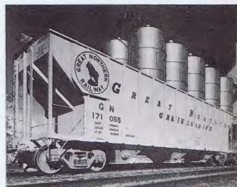
EQUIPMENT ordered includes 500 covered hopper cars with nearly double the grain capacity of a conventional box car.
