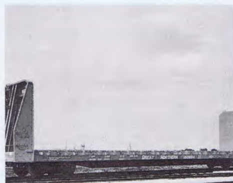
ONE hundred 70-ton bulkhead flat cars equipped with tie-down chains and cushioning devices have been ordered.
