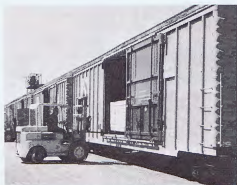
THIS year, GN will take delivery on 300 all-steel, single-sheathed box cars with wide doors for easy loading.
