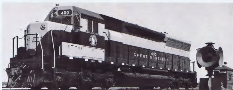
EIGHTEEN new 3,600-horsepower diesel locomotives, similar to the SD-45 shown above, have been ordered from General Motor's EMD Division for delivery this year.
