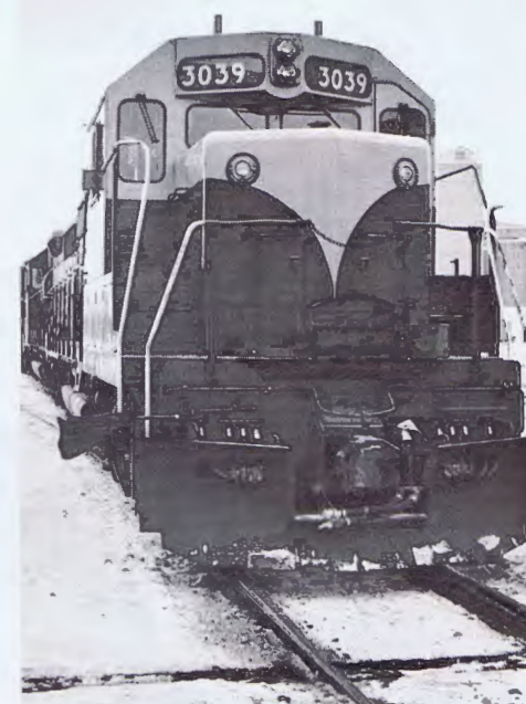
SD-45 locomotive No. 3039, equipped with automatic radio controls, served as the control unit for booster unit 474-B.
