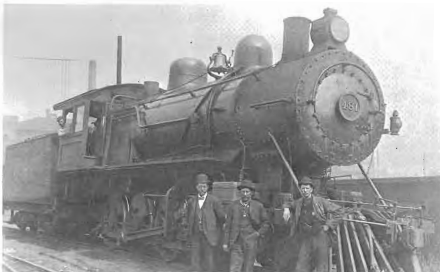
Consolidated "C". Built at the Milwaukee Shops in 1905, this Class C1 2-8-0 Consolidated type had 50-inch driving wheels, weighed 177,000 pounds and put out a tractive effort of 41,120 pounds. Nearly 250 Consolidateds served on the Milwaukee pulling both main and branch line freight trains. Engine 481 was scrapped in September, 1940.
