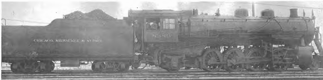
Mikado "L". For more than 30 years the Mikados were the workhorses on the Milwaukee Road's freight trains. Engine 8389 is a Class L2-b Mikado 2-8-2 and is shown here in 1927. Built by Baldwin in 1923, 8389 was not scrapped until December, 1955. These engines were easy to build and maintain. By 1920 more than 10,000 Mikados were in service in the United States, and in 1923 the Milwaukee's Mikado fleet reached 500.
