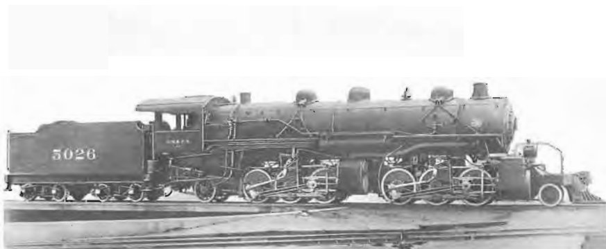
Mallet "N". Designed for steep grades, the 2-6-6-2 Mallet types used by the Milwaukee Road were big, powerful and slow. A Class N2 engine such as 5026 was over 88 feet long, had 57-inch drivers and put out a tractive effort of 70,396 pounds. Combined weight of engine and tender was over half a million pounds. Mallets were primarily intended to pull a 900-ton train at speeds of 6 to 8 miles per hour up the 2.7 per cent grade on the west side of Snoqualmie Pass in Washington, prior to the 1914 completion of Snoqualmie Tunnel. The Mallet's poor performance in winter cold made electrification of the mountain territories a welcome event for engine crews.
