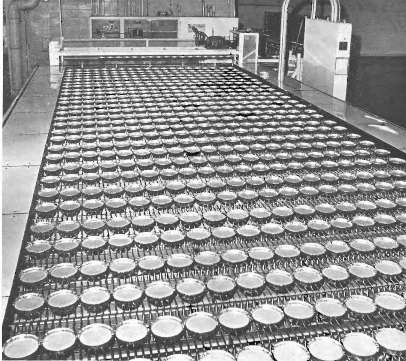
Cream cheese cakes, one of the most popular products in the Sara Lee line, proceed from one of the ovens toward the blast freezer. Refrigeration is powered by gas turbines similar to those used on jet aircraft.
