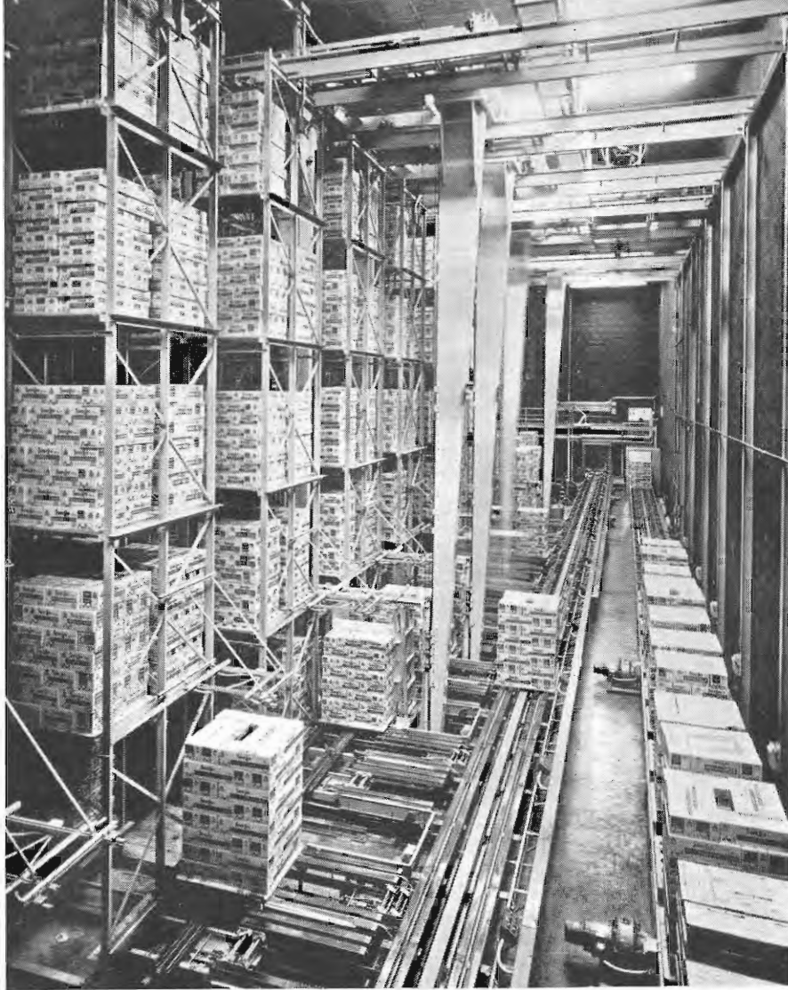
The giant holding freezer, focal point of Sara Lee's revolutionary material handling system. On command from the computer, stacking cranes not only store pallet loads of cartons by variety, but retrieve them to fill orders.
