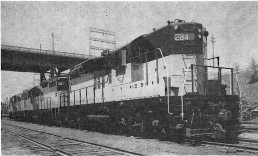
Three new GP-9 diesel electric locomotives coupled together form a solid unit of 5,250 horsepower. Since each has its own operating controls, they may be coupled in multiples to provide whatever power may be needed for freight, passenger or switching service.
