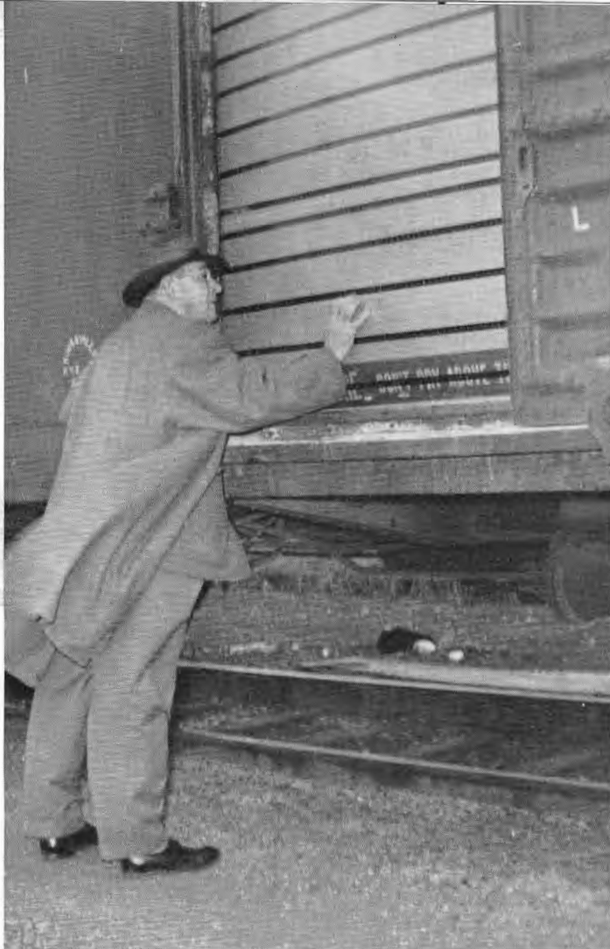
S. M. YATES . . . whose territory is the Chicago Terminal area, closely inspects a paper grain door as the carload of grain stands on the inspection track at Bensenville.
