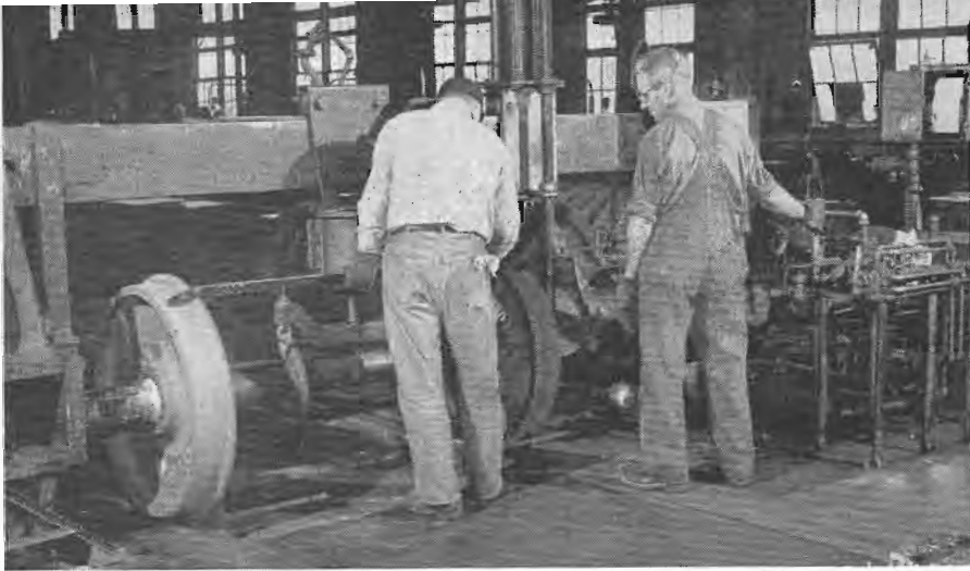
Machinists Norman Ingvaldson and Harold Ellis install new steel wheels of the type which are completely replacing cast iron wheels on Milwaukee Road freight cars. Picture taken in the freight car shop, Milwaukee.
