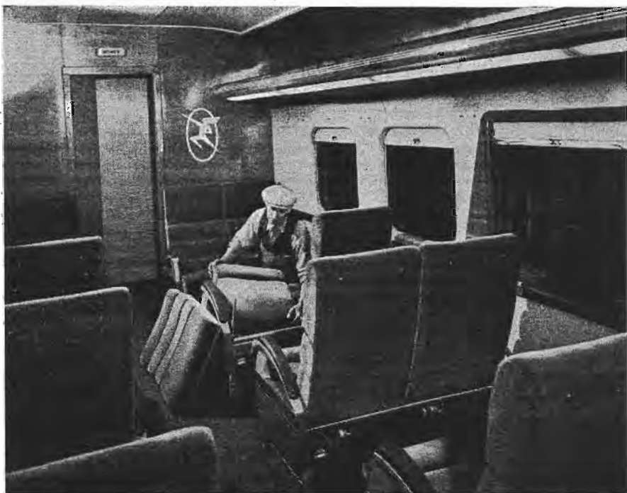
Herbert Bubolz, upholsterer helper, sets the last of the cushions into place in one of coaches. The seat frames were purchased, as was the air foam rubber for the cushions, but all of the upholstering was done in the shops. These seats can be swung around, in pairs, to any desired position. The window units consist of heat-absorbing glass on the outside and shatterproof glass on the inside and are mounted in rubber. Window sills and other wood trim is walnut. The light trough shown is temporary and will be replaced as the car undergoes its final trimming.
