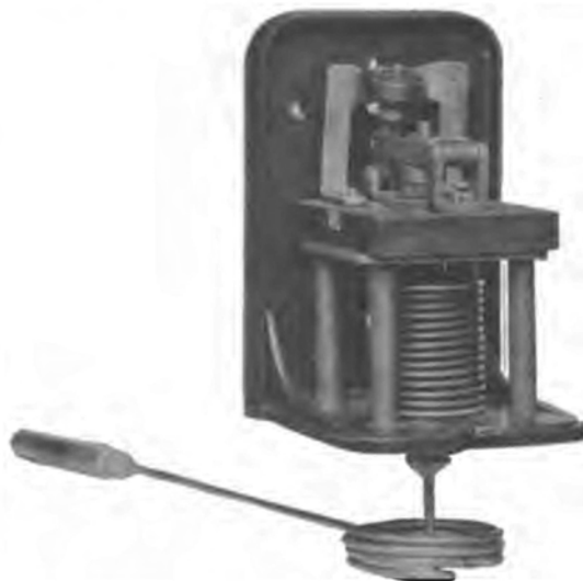
Fig. 24. Temperature Relay, with Cover Removed, used for Protection against Hot Bearings in Automatic Generating Stations
