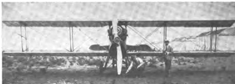
Fig. 15. Biplane Equipped with a G-E Supercharger which can be seen back of the upper blade of the propeller
