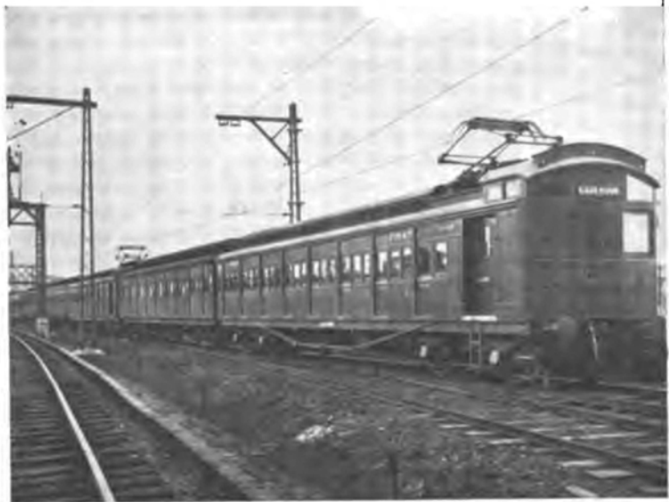
Fig. 17. 1500-volt Direct Current Multiple Unit Train on Victorian Railway, Melbourne, Australia
