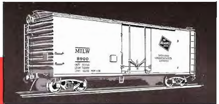
Insulated compartmentizer car
