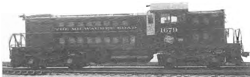
One of two 1,000 H.P. Diesel road switchers, for combination branch line road and terminal switching service.
