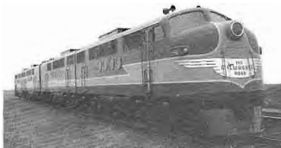
The 5,400 H.P. Diesel freight locomotive to handle the freight service between Avery, Idaho, and Othello, Washington, between our two electrified sections.
